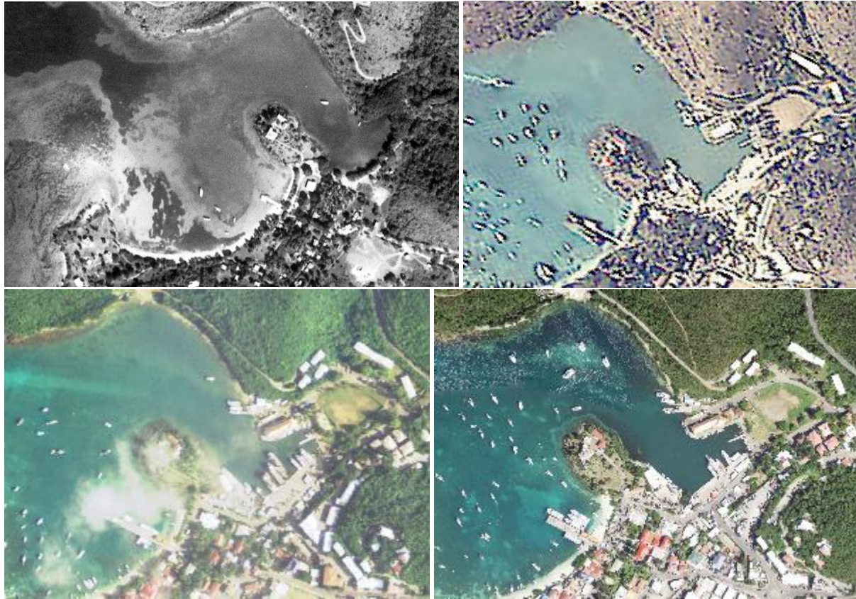
Figure 32: Crux Bay in 1954 (top left), 1980s (top right), 2000s (bottom left), and 2020s (bottom right). Also, in the early 2000's the Car Ferry Dock was built where a sand barrier between the sea and Large Pond was opened (Figure 33). The pond was partially filled, dredged, and opened to the sea.
