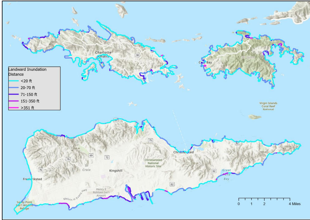
Figure 12: Landward inundation distances expected by tidal flooding assuming a 1 ft sea-level increase
