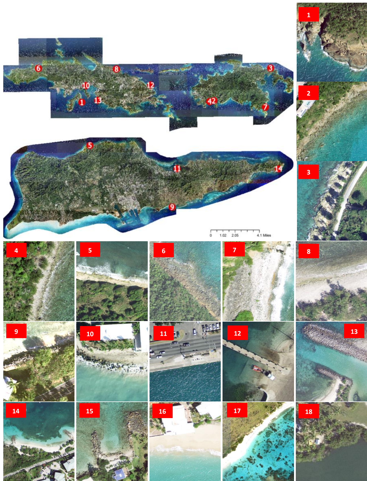
Figure 2: Aerial imagery of different shoreline types. Shot 1: High rocky cliff (rank 1); shot 2: medium erodible cliff (rank 2); shots 3 to 6: Low erodible cliff (rank 3); shot 7 and 8: gravel beach (rank 4); shot 9 and 10: riprap revetment (rank 3 or 4); shot 11: bulkhead or seawall (rank 1); shot 12: pier and boat ramp (rank 1); shot 13: jetty built with riprap (rank 2 to 3); shots 14 and 15: groin built with riprap (rank 2 to 3); shots 16 and 17: sandy beach (rank 5); shot 18: vegetated shoreline (rank 5).
