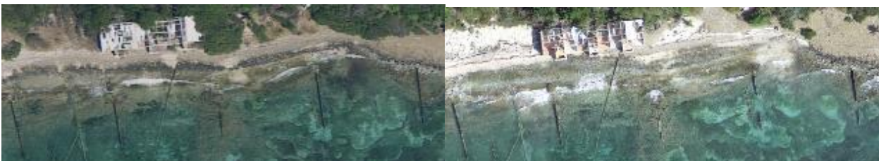
Figure 45: Groins west of the Grapetree Bay Hotel and Villas did not prevent erosion at this location (2010 on the left, 2020 on the right).
